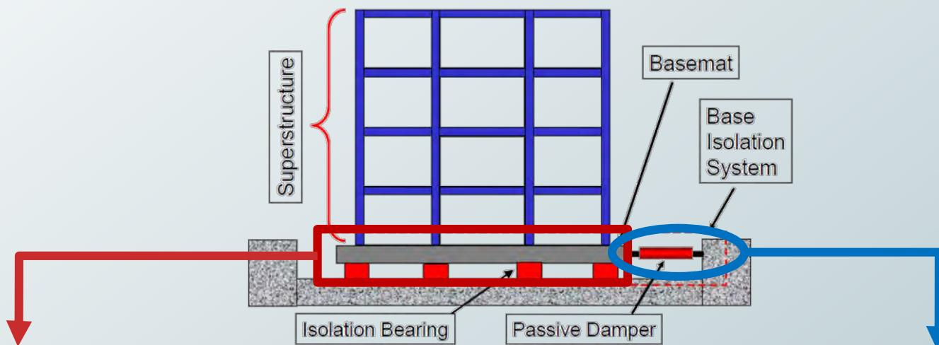
**Effect of Seismic Isolation (ADRS Perspective)**
