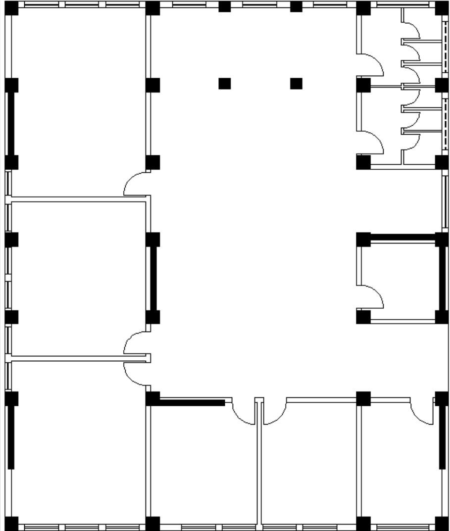
RC shear walls carry earthquake loads down to the foundation. They provide large strength and stiffness to buildings in the direction of their orientation.
