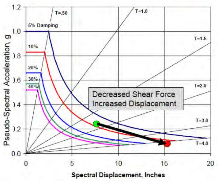
**Effect of Seismic Isolation with Supplemental Dampers (ADRS Perspective)**
