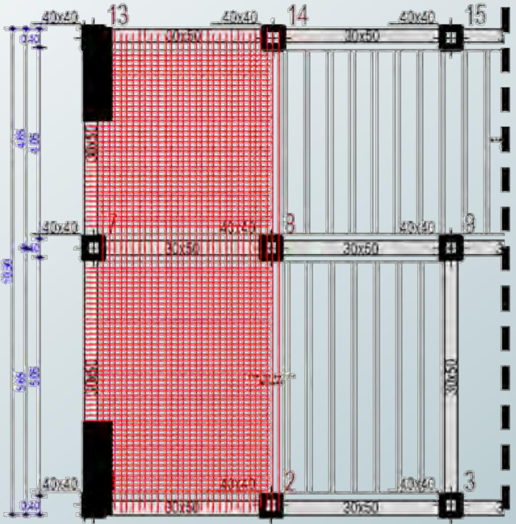
RC floors transmits the actions at columns and walls. Before the intervention the actions are almost distributed and diffused on the floor.
