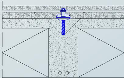
Slab on the top (increasing of stiffness, but also loads)
