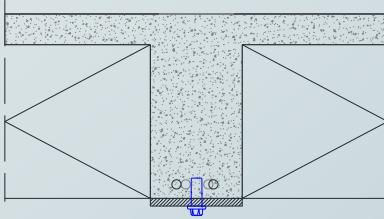
Steel plates in tension, joined with mechanical anchors
